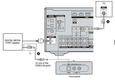
\* The type of connector varies depending on the DIGITAL MEDIA PORT adapter. For details, see the operating instructions supplied with the DIGITAL MEDIA PORT adapter.
